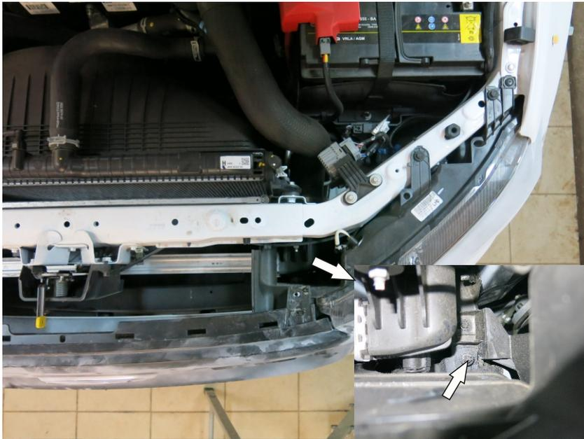
8. Remove 2 screws out of radiator grill.
