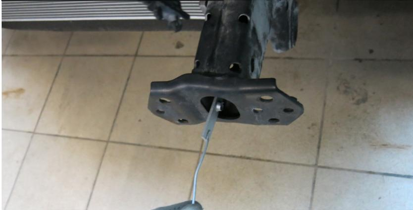
15. Insert nuts (5) into the underframe.
