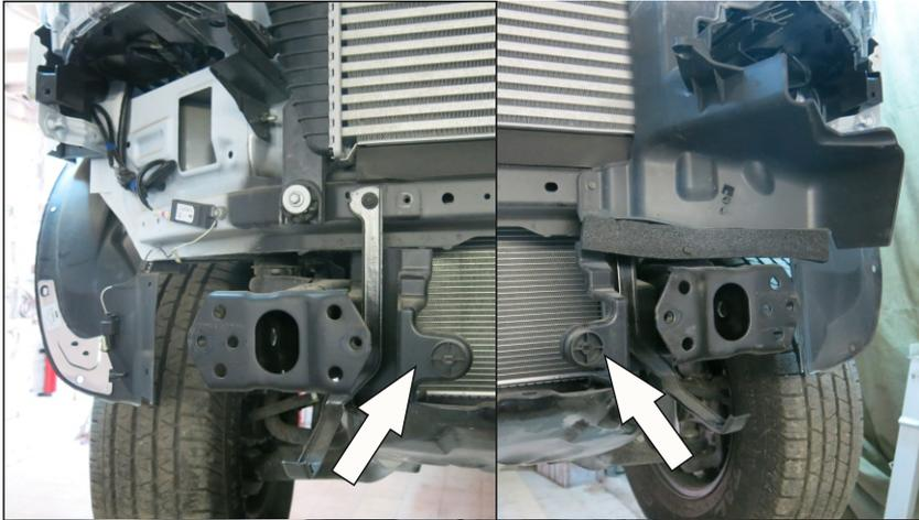
14. Remove plastic dusters from left and right sides of the vehicle.
