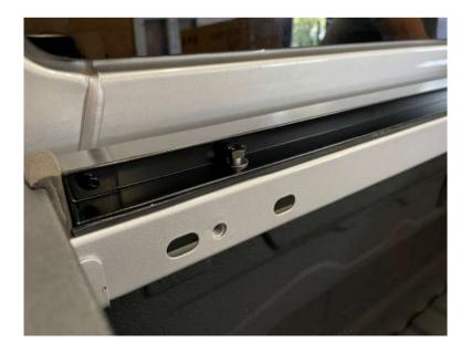
Fasten the U-profile with the supplied M8 screw. Note: We recommend to use Loctite 243 threadlocker.
