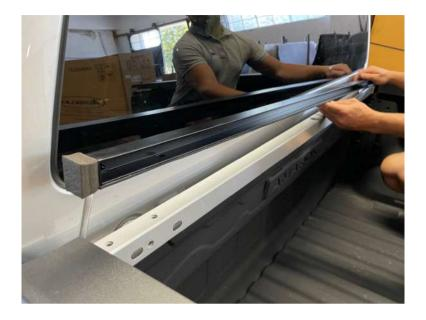
Clean the upper edge of the truck bed in order to have a clean and even surface. Place the aluminium U-profile onto the bulkhead of the truck bed.
