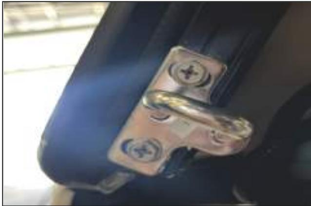
2. Pull the rear hatch down slowly and check the position of the striker in the latch
